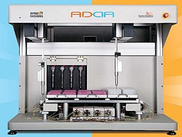
8 seconds per injection, 8 injection ports, no compromises The new ADDA System: an autosampler built for **discovery**.
